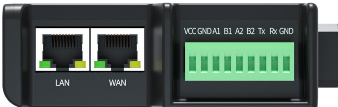
EG8200Mini-104 Interface Identification-1
