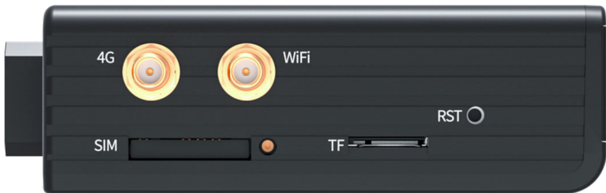
EG8200Mini-104 Interface Identification-1
